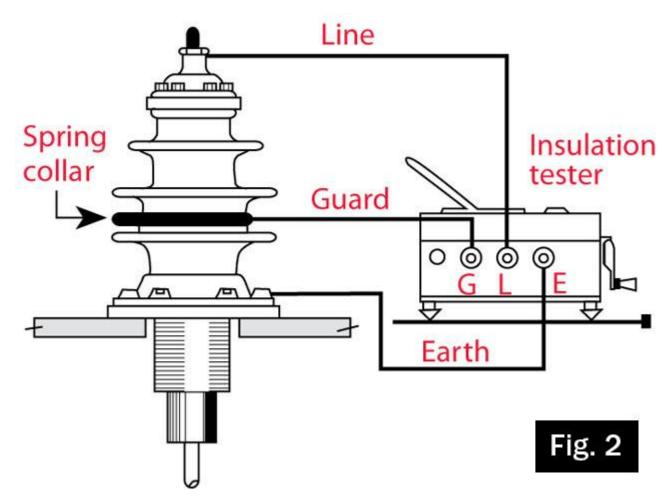
**Figs. 2, 3, and 4** show connections for testing three common types of equipment. Fig. 2 shows a connection for testing a transformer bushing, without measuring the surface leakage. Only the current through the insulation is measured, since any surface current will be returned on the "GUARD" lead.
